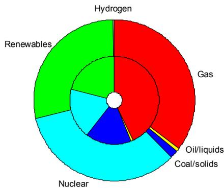
Figure 4.1 *Electricity generation mix in the EU-25 in 2030; baseline (inner circle) compared to Renaissance & Carbon value case (outer circle)*
