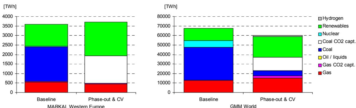
Figure 4.4 *European and global power generation mix in 2050; Phase-out & CV case*
