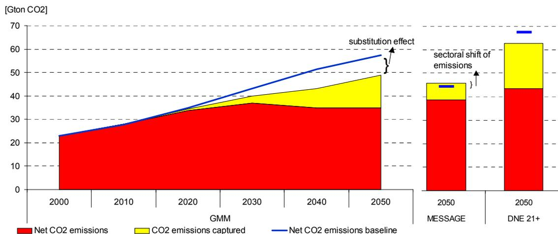
Figure 5.2 Global net CO<sub>2</sub> emissions and amount of CO<sub>2</sub> captured in the CCS Standards case compared to net CO<sub>2</sub> emissions in the baseline
