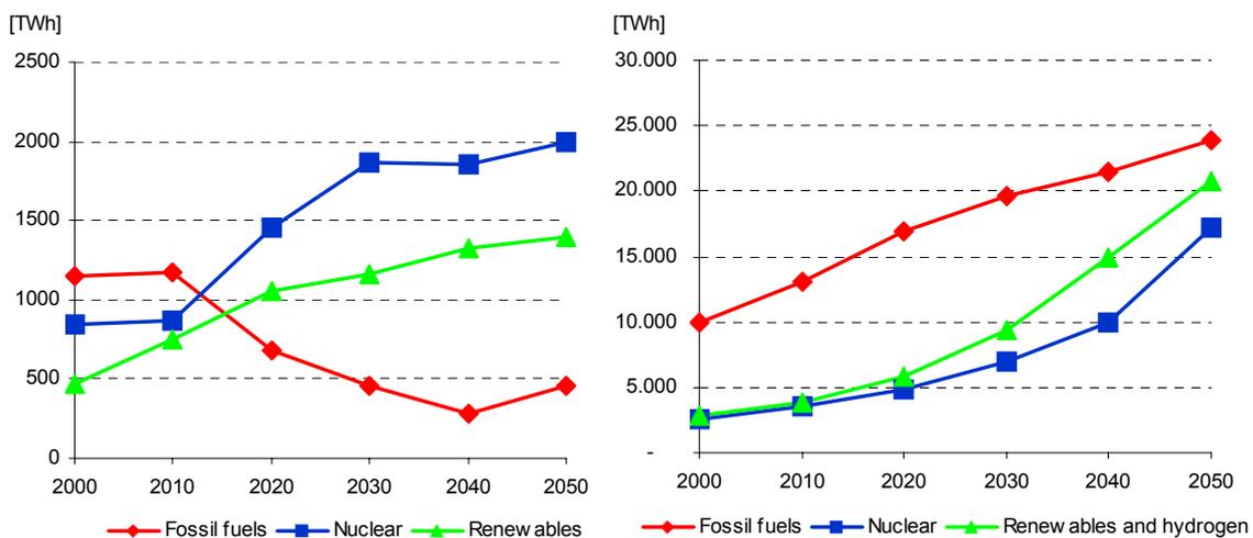
Figure 4.2 *Electricity generation by fuel for Europe and the world for the Renaissance & Carbon value case*
