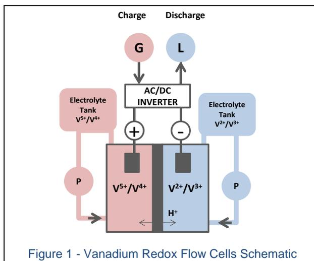
Figure 1 - Vanadium Redox Flow Cells Schematic
